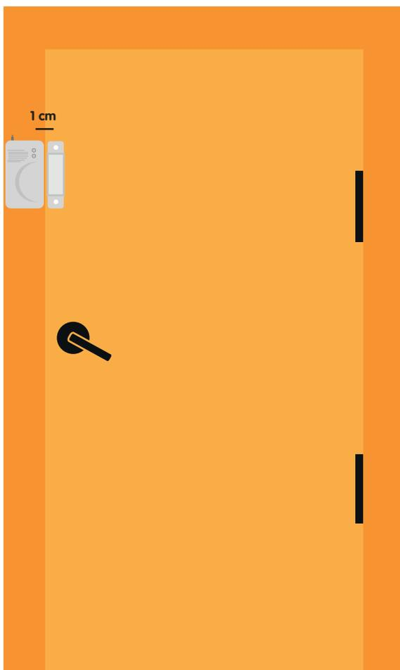
The two items of the device must be aligned and the maximum deviation between them must not exceed 1 cm. (It is sometimes adequate to add wedges – these wedges are not provided).
