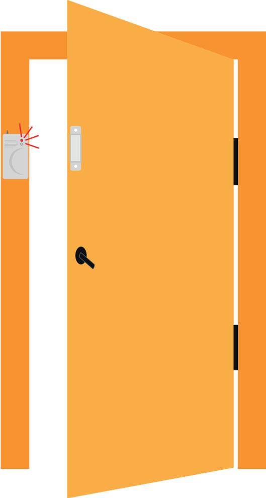
If it doesn't, please check that the distance between the two items is inferior to 1 cm and/or put the main part of the device (with the battery) the other way round (180 rotation)
